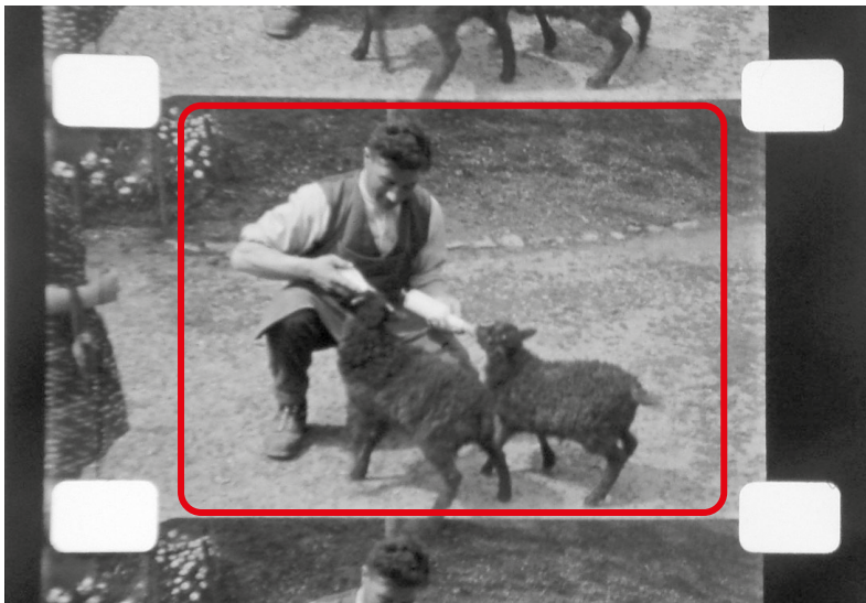
Fig.21: This is 16 mm film that was scanned edge to edge. Due to the shape of the camera's film gate, the film was exposed nearly across its whole width. The red line shows the crop that will be visible during projection.
